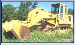
Cat 973 track dozer loader w/ 4 yard bucket, cab, 3,676 hrs. indicated on tach, ser. #90L00443
